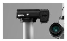
SCM660 Imaging System External Camera Interface Adaptation, Canon and Sony cameras.
